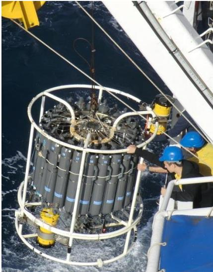
At every station, pressure (P), salinity (S), potential temperature ( $\theta$ ) dissolved oxygen concentration (DO) and fluorescence were measured with a CTD-rosette system consisting of a CTD SBE 911 plus, and a General Oceanics rosette with 24 Niskin Bottles (12 liters each).
