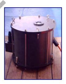
Measurement of bio-optical parameters using the PUV Biospherical 510B profiler
